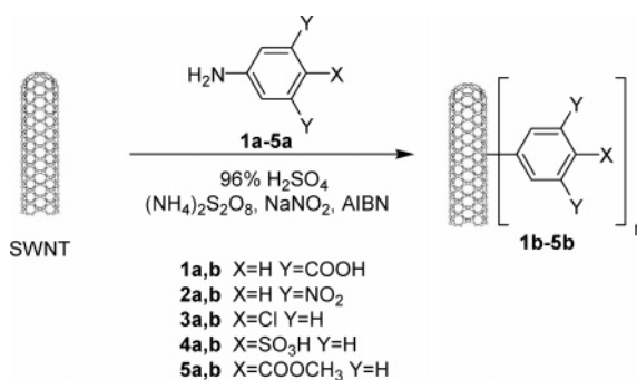
Scheme 1. Functionalization of SWNTs with Aniline Derivatives in 96% \text{H}_2\text{SO}_4 and Ammonium Persulfate
